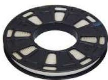
Trim a wide variety of coatings, from medium durometer polyurethane to high durometer polyureas; Medium-tack adhesive, developed for applications where less adhesive strength is preferred; Contains a .010" diameter, high-tensile metal wire filament; Over 50% more cutting strength than our Standard strength product; Used for thicker, harder, and aggregate-filled coatings
